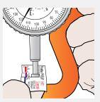
1.Tear off one section of the 2. Stick the tape on to the test 3. Using a micrometer such tape from the roll, peel off the surface, and rub the central as the Elcometer 124 Foil backing tape and retain the portion using the swizzle stick Thickness Gauge, measure the thickness of the central pencil or similar rounded object portion of the tape replica and substract 50µm (2mils) from the reading. This result is the peak-to-valley profile height. Write the value on the tape.
